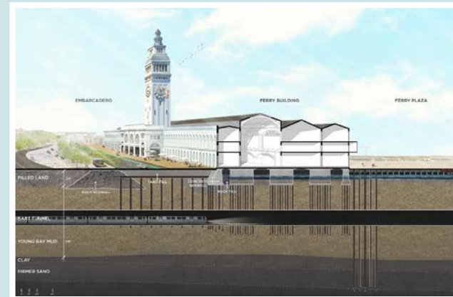
Cross-Section of Ferry Building Substructure
