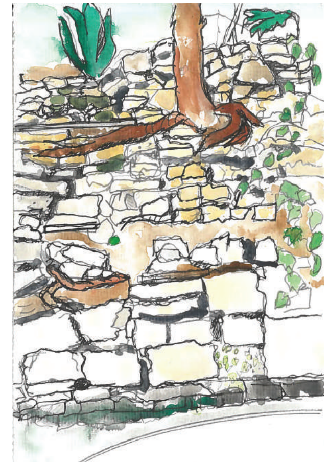
Perspective drawing of portion of wall with root intrusion.
