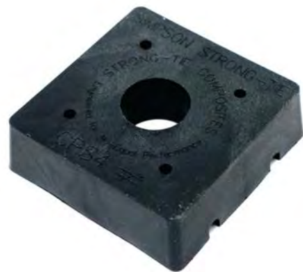
Simpson Strong-Tie connector. The CPS is a composite plastic standoff designed for increased concrete surface area. It also keeps moisture away from the bottom of the post. Install with 10d common nails and 5/8 in. Dia anchor bolt.
